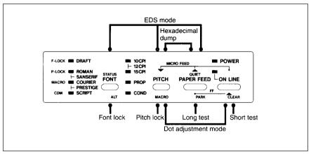
Figure 4-2. Power-up functions of control panel.
