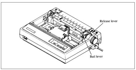
Figure 7-2. Remove the front cover, and move the bail lever toward the front of the printer.
