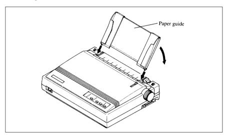
Figure 2-9. Installing the paper guide.
