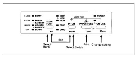
Figure 5-1. Button functions in the EDS mode.
