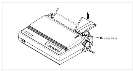
Figure 3-9. Tear off the printed fanfold paper.
