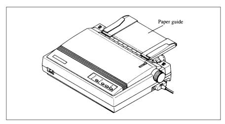
Figure 3-7. Close the rear cover, then set the paper guide horizontally.
