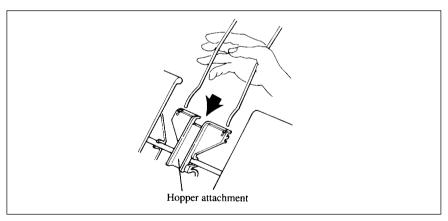
Figure 7-5. Insert the hopper attachment.
