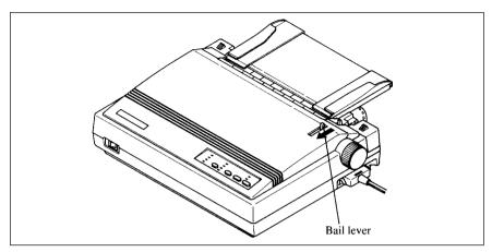
Figure 3-8. Pull the bail lever toward the front of the printer to load paper.
