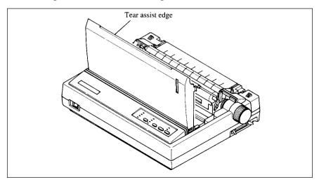
Figure 2-4. The front cover can stay on the printer.
