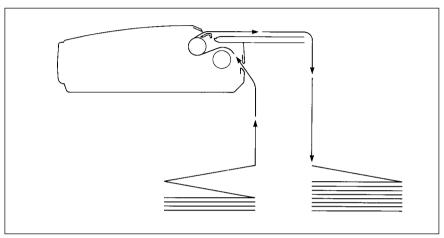
Figure 3-3. Paper path for fanfold forms.
