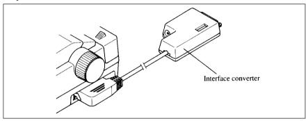
Figure 7-11. Connect the Parallel connector to the printer.
