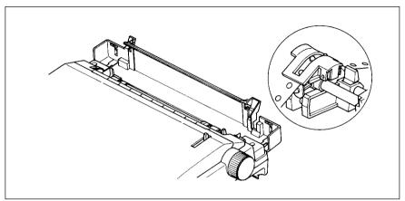
Figure 3-6. Adjust the tractor positions to accommodate the width of fanfold forms.
