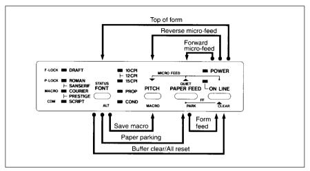
Figure 4-5. Switch combination functions of control panel.
