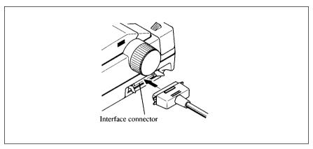
Figure 2-10. Connecting the interface cable.
