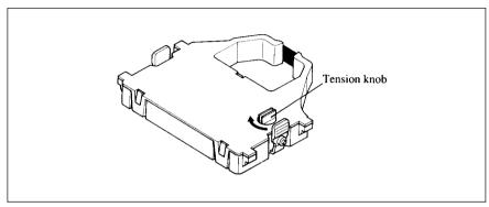
Figure 2-5. Take out the slack of the ribbon by turning the tension knob on the ribbon cartridge.
