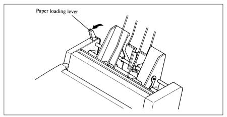
Figure 7-7. Pull the paper loading lever forward.
