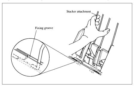
Figure 7-6. Insert the stacker attachment.
