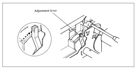
Figure 3-2. Location of the adjustment lever.
