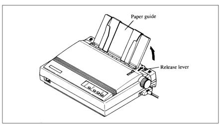
Figure 3-11. Raise the paper guide for single sheets.
