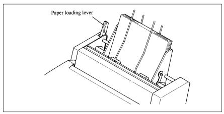
Figure 7-10. Push the paper loading lever to hold the paper stack.
