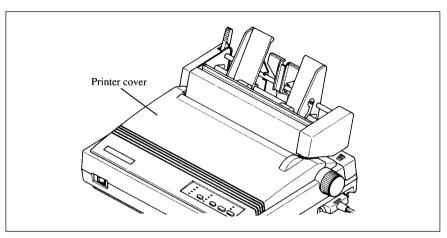
Figure 7-4. Install the printer cover.
