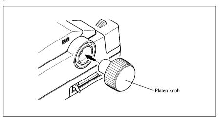
Figure 2-2. Installing the platen knob.
