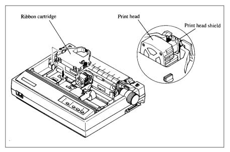
Figure 2-6. Installing the ribbon cartridge.
